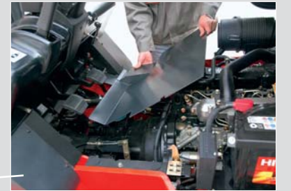
Easily-Detached Floor Panel One-touch removal of the floorboard gets you right to service operations and reduces down-time.
